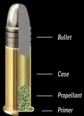
All four components of a rimfire cartridge are strenuously monitored in every stage of production and then coordinated perfectly prior to loading (placing the charge in the ammunition). This is the only way to guarantee maximum precision and reliability across different manufacturing batches.
